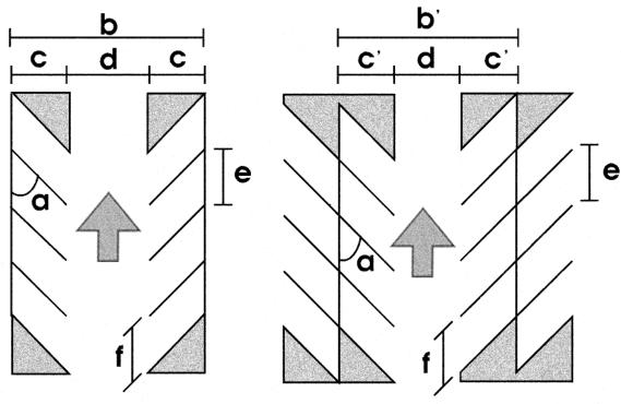
a Parking Angle b/b' Parking Section Width c/c' Parking Bank Width d Aisle Width e Curb Length Per Car f Car Stall Width
