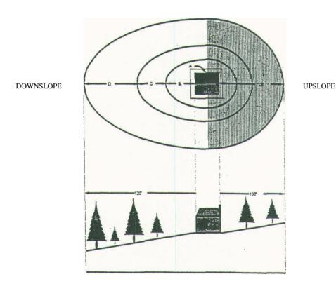
The shaded areas (unsloped) of B, C, & D remain a constant distance of 10', 20', and 70' respectively. The shaded area begins from the mid-section of a structure. The unshaded areas (downslope) of B, C, & D increase with slope as detailed below:
