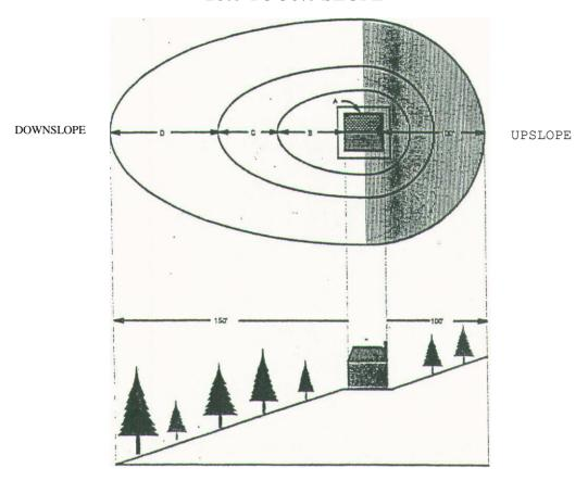
The shaded areas (upslope) of B, C, & D remain a constant distance of 10', 20', and 70' respectively- The shaded area begins from the mid-section of a structure. The unshaded areas (downslope) of B, C, & D increase with slope as detailed below:
