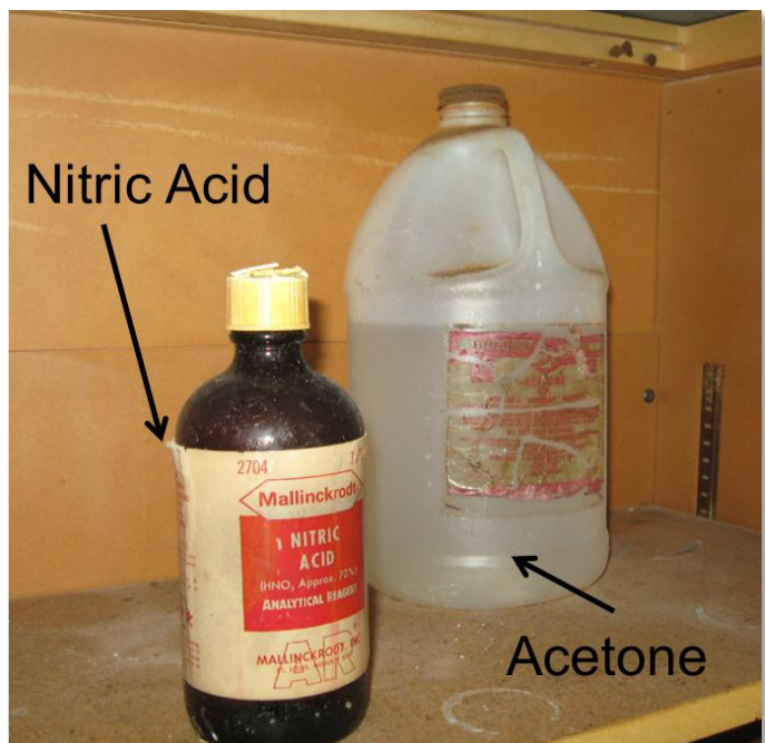
Figure 15 - photo of Nitric Acid and Acetone in a cabinet in a school in Montana. Concentrated Nitric Acid mixed with organic solvents results in violent explosions.
