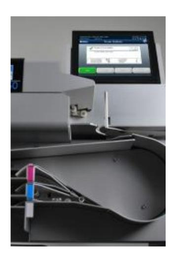
The Models DS450/DS850/DS950 Tabulators are high-speed optical and digital scan central paper ballot counter and vote tabulators which have the capacity to route ballots to different bins depending on selected criteria (write-ins, overvotes, blank ballots).
