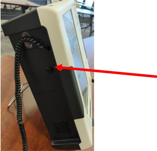
5. Use the medium barrel key to lock the right-side paper path access door.
