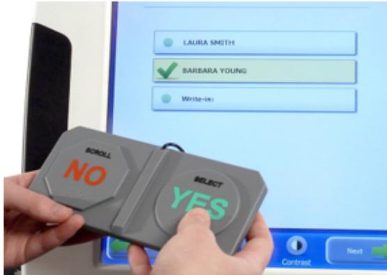
The rocker switch is a large-button, two-position switch assistive technology that can assist [voter's](#) who are unable to use the ExpressVote touch screen or the audio-tactile keypad. The rocker switch device can be hand-held, placed on a table, or placed on the floor for foot operation.
