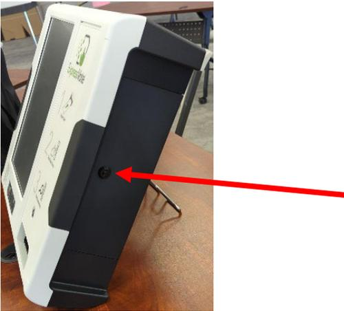
6. When the ExpressVote® is configured on a standard table, secure the rear USB port by affixing a tamper-evident label seal as noted below in the photo.
