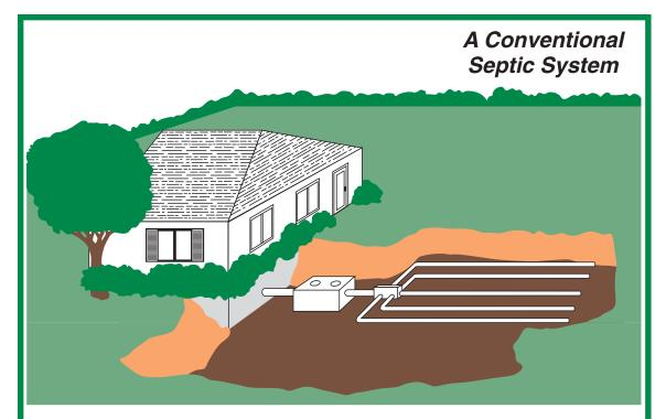
A septic system consists of a septic tank, a distribution box and a drainfield, all connected by pipes, called conveyance lines.
