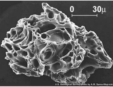
Figure 4-93 Microscopic View of Volcanic Ash
